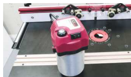
▲ The Mast-R-Lift Excel II lift is designed for the AUK router but is sold as a separate item
